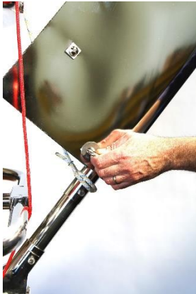
Figure 4 - Place eyebolt through upper holes in e-rudder foil. They should be clear of Monitor water paddle allowing eyebolt to pass through.
