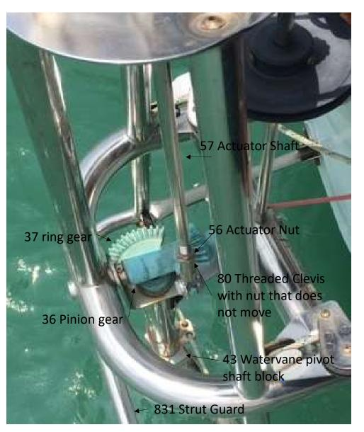
To re-align the gears:
