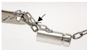
Attach tether chain to anchor chain with short Velcro strap.
