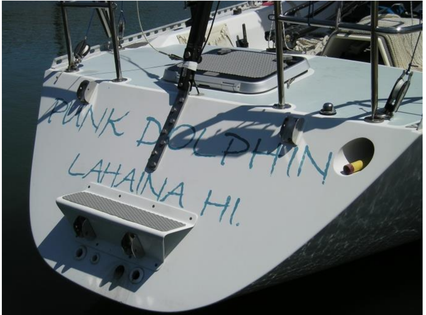
The transom of the Wylie 39 "Punk Dolphin". The upper mounting brackets are on the transom, and the lower mounting brackets can be seen on the after face of the step near the bottom of the transom.
