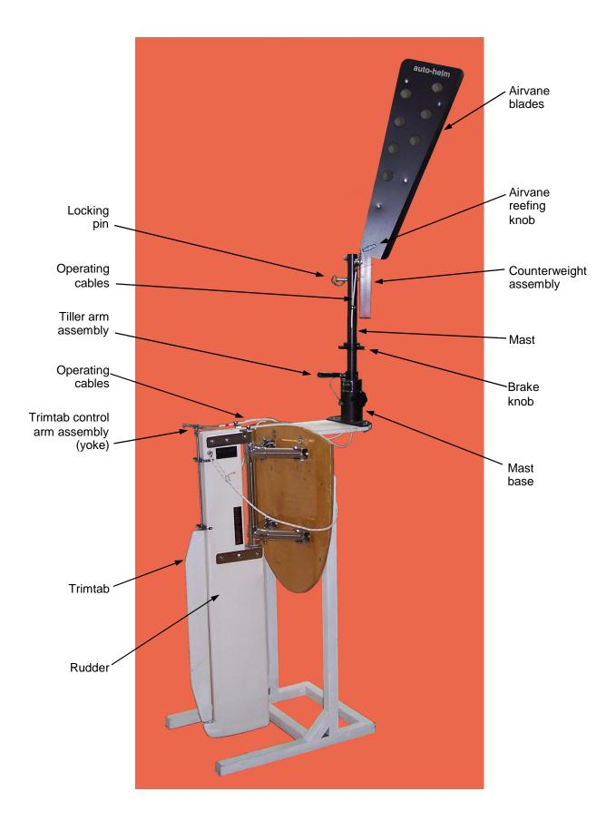
the boat. The Auto-helm is capable of steering boats up to approximately 48 feet LOA. The rudder is a heavy fiberglass shell filled with high density polyurethane closed cell foam. This makes for a strong rudder which is also buoyant. Due to the buoyancy of the rudder, the Auto-helm's true weight is only 32 lb. Shipping weight is approximately 98 lb. The rudder supports are 316L stainless steel, and there is no metal in the water.
