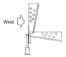
It is important to remember which windvane edge is the leading edge and which is the trailing one. It is possible to bring the vane upright by turning the back edge into the wind, but this will produce completely reversed reactions in the vane gear taking the boat further off course instead of bringing it back to the desired heading.
