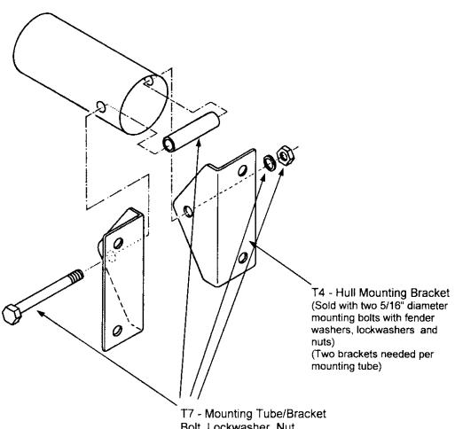
I / - Mounting Tube/Bracke Bolt, Lockwasher, Nut & Compression Tube
