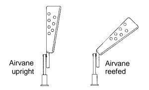
The counterweight under the airvane balances the vane. Ideally, it should barely be able to keep the vane upright when there is no wind. The airvane must not be top heavy. Without the counterweight keeping the airvane upright, it would not work at all.
